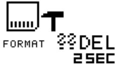
To confirm and start the formatting process, press the DEL button for at least 2 seconds. If you want to cancel the formatting process, either remove the memory card or move the 4-Position Switch.
